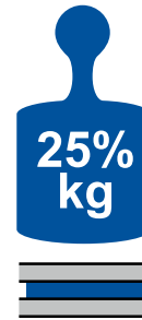
Horizontally mounted = 25% quoted load rating
